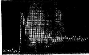
FIGURE 37—30V Protector Vertical: 20V/div.; Horizontal: 10nsec/div.
